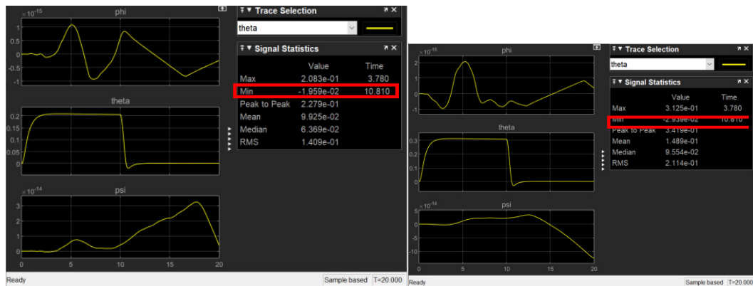
Figure 12 shows the Euler angle variations for different conditions: a step response termination value of 0.2 and a pulse function magnitude of -10, and a step response termination value of 0.3 and a pulse function magnitude of -15.
